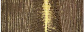
In traditional filter design, the pleats are often pinched closed. The clean area seen on the inside of these pleats indicates that the dirty air never reached this media, resulting in less effective loading and ineffective pulse cleaning and as a result, short filter life.
