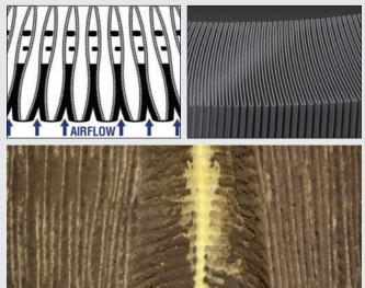
In traditional filter design, the pleats are often pinched closed. The clean area seen on the inside of these pleats indicates that the dirty air never reached this media, resulting in less effective loading and ineffective pulse cleaning and as a result, short filter life.
