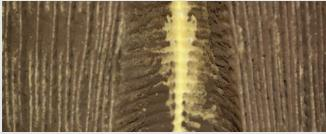
In traditional filter design, the pleats are often pinched closed. The clean area seen on the inside of these pleats indicates that the dirty air never reached this media, resulting in less effective loading and ineffective pulse cleaning — and as a result, short filter life.
